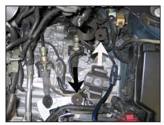
10. Remove the two air filter housing mounting grommets shown.
