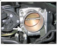
11. Remove the lower front throttle body mounting bolt shown. This bolt will be reused in the next step.
