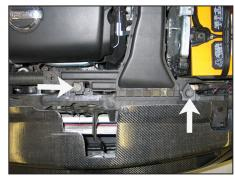
4. Remove the two bolts that secure the fresh air intake duct to the core support. These two bolts will be reused in a later step.
