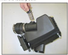
23. Remove the two screws securing the mass air sensor, then remove the mass air sensor from the stock airbox as shown.
