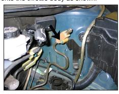
13. Remove the slave cylinder bleeder bolt shown. NOTE: Vehicles equipped with an automatic transmission will not have a bolt in this location.
