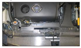
22. Reinstall the fresh air intake scoop and secure with the factory bolt.
