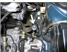
18. Install the shorter rubber mounted stud onto the rear airbox mounting bracket as shown.
