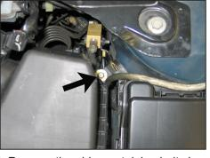
8. Remove the airbox retaining bolt shown. **NOTE: This bolt is located at the rear of the airbox near the strut tower.**
