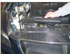
3. Remove the fresh air intake scoop from the vehicle as shown.
