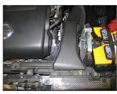
21. Reinstall the intake duct onto the core support and into the heat shield assembly. Secure with the factory bolts.
