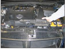
5. Remove the fresh air intake duct from the vehicle as shown.
