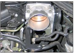
12. Using the bolt removed from the previous step, install the provided tube mounting bracket (070113) onto the throttle body as shown.
