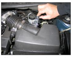
7. Disconnect the mass air sensor electrical connection.
