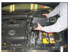
9. Loosen the hose clamp, which secures the intake tube to the throttle body. Remove the complete stock intake assembly from the vehicle. NOTE: K&N Engineering, Inc., recommends that customers do not discard factory air intake.
