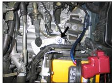
19. Install the longer rubber mounted stud onto the front airbox mounting bracket as shown.
