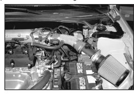
42. This intake kit has been designed to be used in two different configurations. In the case of inclement weather, the cold air tube can be removed and the air filter can be clamped onto the intake tube located in the engine compartment to avoid the possibility of ingesting water into the engine. NOTE: If you have any concerns, return the
