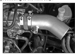
23. Install the throttle body tube onto the throttle body as shown, but do not tighten at this point.
