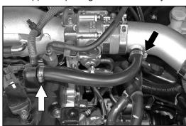
38. Install the provided vent hose onto the cam cover and the intake tube and secure with the provided hose clamps as shown.
