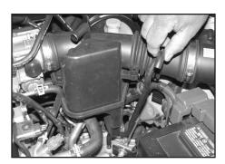
5. Remove the transmission vent hose from the resonator as shown.
