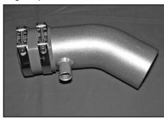
22. Install the silicone hose and hose clamps onto the throttle body tube and tighten as shown. NOTE: Before installing the silicone hose, inspect the inside of the tube for any debris, then clean the inside out with water and a towel. Inspect the tube one more time before proceeding to the next step.
