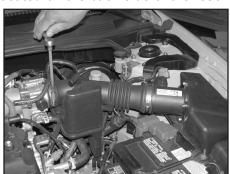
6. Loosen the hose clamp at the throttle body as shown.
