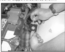
26. Install the larger flat washer and rubber fender washer to the bottom side of the air cleaner support bracket as shown. Install the rubber mounted stud and another flat washer and secure from underneath with the provided nylock nut.
