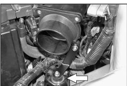
28. Secure the bracket to the rubber mounted stud using the provided hardware as shown.
