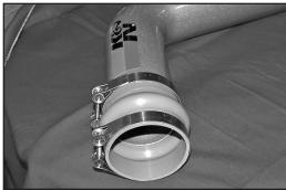
29. Install the stepped hump hose onto the cold air tube and secure it with the provided hose clamps as shown.
