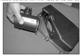
19. Loosen and remove the four bolts that secure the mass air sensor, then, remove the mass air sensor as shown.
