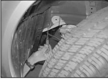
15. Remove the push clip from the inner wheel house valance as shown.
