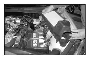
11. Pull firmly upwards to release and remove the lower air cleaner assembly as shown. NOTE: K&N Engineering, Inc., recommends that
