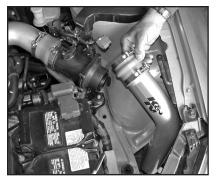
31. Slide the cold air tube into the hole in the inner fender as shown.
