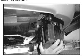
35. From underneath the vehicle install the K&N® air filter onto the cold air tube and secure with the provided hose clamp.
