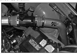
32. Slide the hump hose onto the mass air sensor assembly as shown but do not tighten completely.
