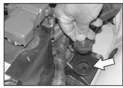
25. Remove the stock rubber grommet from the air cleaner support bracket as shown.
