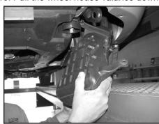
17. From underneath the vehicle, loosen and remove the two bolts that secure the intake resonator, then remove the resonator as shown.
