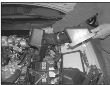
9. Remove the upper air cleaner assembly as shown.
