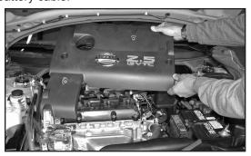
2. Remove the four bolts that retain the engine cover, then remove the engine cover.
