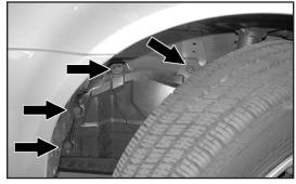
12. Remove the four push clips from the inner fender valance as shown.
