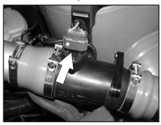
39. Reconnect the mass air sensor electrical connection as shown.
