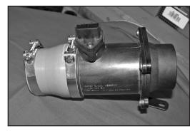
24. Install the silicone hose and hose clamps onto the mass air sensor as shown.
