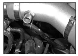
36. Slide the transmission vent hose into the provided wire hanger as shown, then slide the wire hanger onto the vent tube on the throttle body tube as shown
