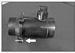
20. Assemble the mass air adapter and the mass air sensor using the provided hardware as shown. NOTE: One of the button head screws is longer than the others and should be placed in the orientation as shown.
