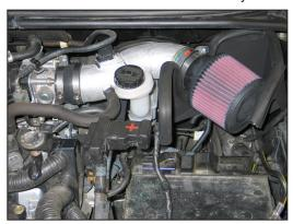
22. Install the K&N® air filter onto the K&N® intake tube and secure with the provided hose clamp.
