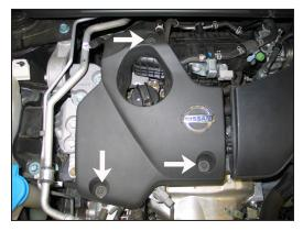
6. Remove the three bolts which secure the engine cover and then remove the engine cover.
