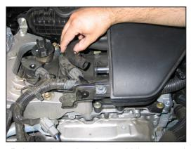
7. Release the spring clamp which secures the crankcase vent hose to the intake plenum and then disconnect the crankcase vent hose.
