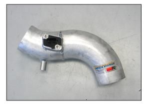
14. Install the mass air sensor into the K&N $^{\odot}$  intake tube and secure with the provided hardware.
