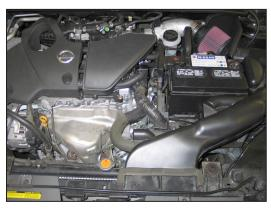
27. Reinstall the engine cover and secure with the factory bolts.
