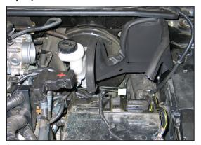
16. Secure the heat shield to the inner fender using the provided hardware.
