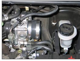
19. Install the silicone hose (084036) onto the throttle body and secure with the provided hose clamp.
