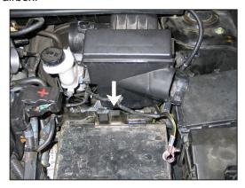
11. Remove the airbox mounting bolt located below the wiring harness, between the battery tray and airbox.
