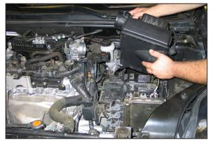
12. Remove the airbox from the vehicle.
