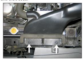
2. Remove the two retaining clips which secure the fresh air supply duct to the core support.
