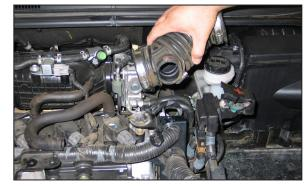
9. Loosen the hose clamps which secure the intake tube and then remove the intake tube from the vehicle.
