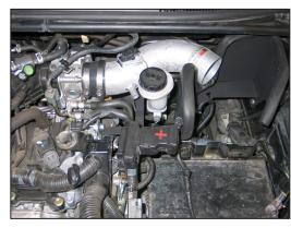
20. Install the K&N® intake tube into the silicone hose on the throttle body and align with the mounting bracket installed in step #19. Secure with the provided hardware and hose clamp.
