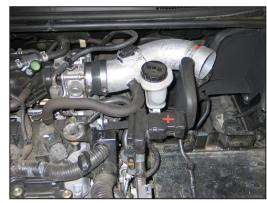
21. Install the crankcase vent hose onto the K&N® intake tube and secure with the factory hose clamp.
