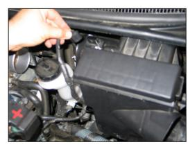
10. Disconnect the mass air sensor electrical connection and then release the harness from the airbox.
