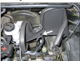
17. Secure the transmission vent hose to the heat shield with the provided tie wrap passing through the hole in the bottom of the heat shield.
