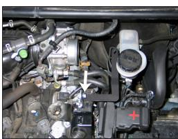
18. Install the intake tube mounting bracket onto the engine lifting bracket and secure with the provided hardware.
