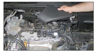
8. Remove the resonator mounting bolt and loosen the hose clamp which secures the resonator to the intake tube. Remove the intake resonator from the vehicle.
