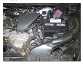
26. Reinstall the intake resonator and secure with the factory bolt.
