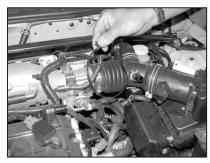
6. Remove the tie-wrap that secures the electrical connection to the rubber intake tube as shown.
