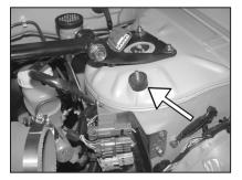
21. Remove the plastic push clip from the strut tower, then, install the provided rubber mounted stud into the threaded hole as shown.
