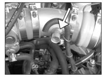
34. Slide the wire hanger onto the vent on the throttle body tube as shown.
