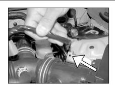
4. Unclip the mass air wire from the bracket on the mass air sensor as shown.
