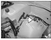
22. Install the provided rubber mounted stud into the threaded hole on the inner fender as shown.
