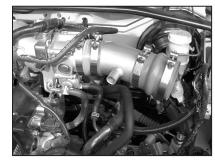
17. Slide the throttle body tube into the silicone hose on the throttle body as shown, but do not tighten.
