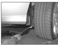
13. Remove the one screw and four push clips on the inner vender valance, then pull the valance down as shown.
