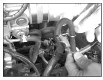
33. Slide the provided wire hanger onto the transmission vent hose as shown.
