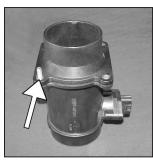
19. Secure the provided mass air adapter to the stock mass air sensor using the provided button head screws.
