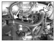
35. Install the provided hose and hose clamps onto the cam cover, then, connect the other end to the vent on the throttle body tube as shown. Tighten hose clamps.
