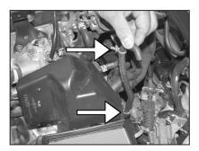
10. Using a pair of pliers, unclip the transmission vent hose from the lower air cleaner assembly as shown.
