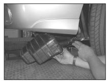
14. From underneath the vehicle loosen and remove the two bolts that secure the air intake resonator, then, remove the resonator as shown.
