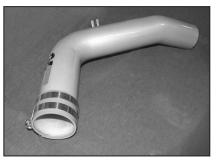
25. Install the silicone hose and hose clamps onto the K&N cold air tube as shown. **NOTE: Before installing the silicone hump** hose, Inspect the inside of the tube for any debris, then clean the inside out with water and a towel. Inspect the tube one more time before proceeding to the next step.
