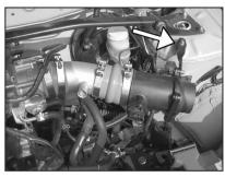
24. Slide the mass air assembly into the hump hose and line up the bracket with the rubber mounted stud on the strut tower and secure with the provided hardware as shown.
