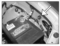
23. Install the remaining rubber mounted stud into the threaded hole on the inner fender as shown.
