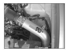
28. Line up the silicone hose on the cold air tube with the mass air sensor adapter, then slide the silicone hose onto the adapter and tighten with the provided hose clamp as shown.
