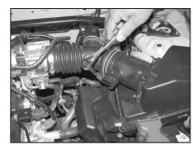
7. Loosen the hose clamp at the mass air sensor as shown.
