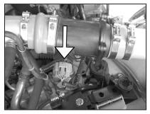
36. Reconnect the mass air sensor electrical connection as shown.
