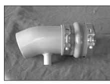
16. Install the stepped hump hose and hose clamps onto the throttle body tube and tighten as shown.
