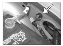
30. Secure the lower bracket on the cold air tube with the rubber mounted stud on the inner fender, then, secure it with the provided hardware as shown.
