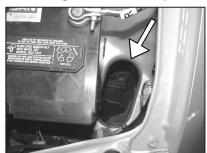
26. Apply the provided edge trim to the hole on the inner fender as shown.
