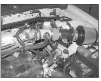
40. This K&N<sup>®</sup> high flow intake system has been designed to be used in two different configurations. In the case of inclement weather, the cold air tube can be removed and the air filter can be clamped onto the intake tube located in the engine compartment to avoid the possibility of ingesting water into the engine.
