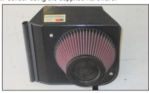
17. Install the K&N® air filter onto the filter adapter and secure with the provided hardware.
