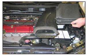
3. Unclip the four upper airbox retaining clips; then remove the upper airbox and fresh air duct assembly as shown.
