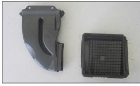
20. Remove the fresh air duct from the upper airbox housing.
