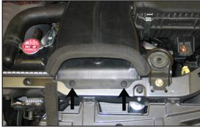
2. Loosen the plastic screws shown which retain the fresh air supply duct.
