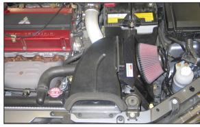
22. Clip the fresh air supply duct onto the heat shield and secure the front with the factory plastic screw.
