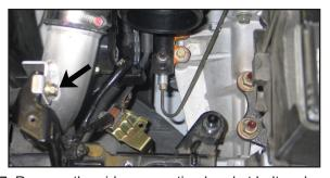
7. Remove the airbox mounting bracket bolt and intercooler mounting bolt shown. Unhook the wiring harness from the airbox mounting bracket; then remove the mounting bracket from the vehicle. NOTE: The airbox mounting bracket bolt will be reused in a later step.
