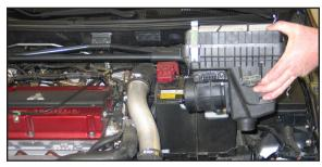
5. Lift the mass air sensor/airbox assembly up, disconnect the mass air sensor electrical connection and unhook the wiring harness from the airbox. Then remove the complete assembly as shown
