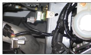
18. Disconnect the solenoid valve electrical connection and reroute the mass air sensor/ solenoid valve wiring harness under the main wiring harness as shown. Reconnect the solenoid valve wiring connection.
