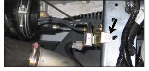
8. Reinstall the solenoid valve in its original location and secure with the factory bolts removed during step #6.
