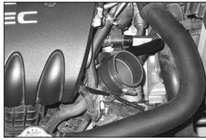
19. Install the provided silicone hose (08284) onto the throttle body and secure with the provided hose clamps.
