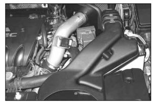
28. Reinstall the fresh air intake scoop and secure with the factory retaining clips.
