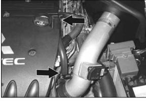
25. Install the provided crank case vent hose onto the 90° barbed fitting on the K&N $^{\textcircled{R}}$  intake tube. Then attach the open end of the vent hose onto the valve cover vent port as shown.
