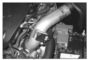
24. Install the K&N<sup>®</sup> intake tube into the silicone hose at throttle body and align with the mounting bracket installed in step #18. Secure the intake tube with the provided hose clamp and hardware. NOTE: It may be necessary to reposition the positive battery cable to obtain proper clearance of the tube.
