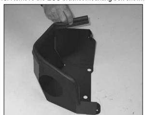
11. Install the long piece of the edge trim onto the heat shield as shown.
