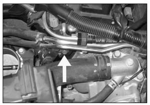
18a. On vehicles not equipped with an EGR tube, remove the bolt shown which secures the steel vacuum lines to the engine.
