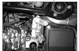
10. Remove the ECU bracket mounting bolt shown.
