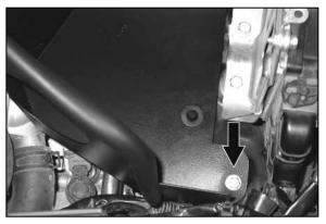
17. Secure the front of the heat shield to the front air box mount with the provided hardware. Tighten all the heat shield mounting bolts.
