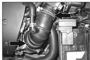
6. Loosen the two hose clamps that secure the stock intake tube to the throttle body and air filter housing.
