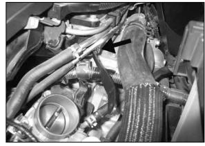
18b. Secure the provided tube mounting bracket (083140) to the engine using the provided hardware.
