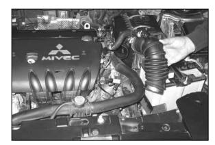
7. Remove the stock intake tube from the vehicle as shown.
