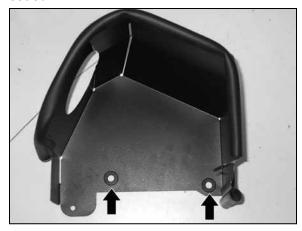
13. Install the two 7/16" ID grommets (08092) that are provided into the mounting holes in the heat shield as shown.
