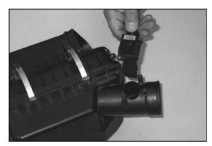
20. Remove the two screws that secure the mass air sensor into the factory air box and remove the mass air sensor as shown.
