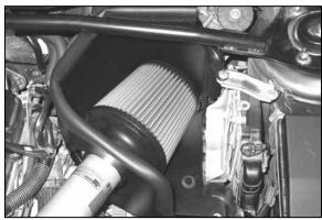
26. Install the K&N<sup>®</sup> air filter onto the intake tube and secure with the provided hose clamp.
