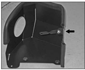
14. Install the heat shield bracket (070702) onto the heat shield as shown.
