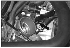
18. On vehicles equipped with an EGR tube, unhook the engine wiring harness from the clip and move the wiring harness rearward as shown. Install the intake tube mounting bracket (06724) onto the intake manifold and secure with the provided hardware.
