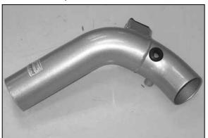
22. Install the provided  $\frac{1}{2}$ "ID grommet (08064) into the intake tube as shown.
