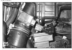
4. Disconnect the mass air sensor electrical connection and unhook the mass air sensor wiring harness from the air box.
