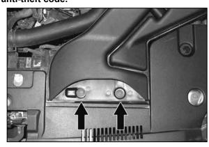
2. Remove the two fasteners that secure the fresh air intake scoop shown.
