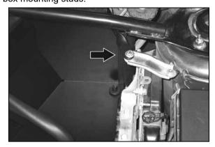
16. Place the supplied spacer under the heat shield mounting bracket and then secure the bracket to the ECU mounting bracket with the provided hardware as shown.
