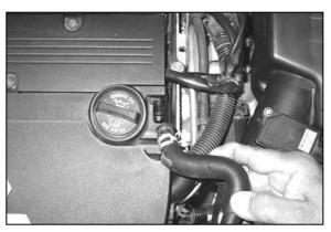
5. Release the spring clamp that secures the crank case vent hose to the valve cover port. Disconnect the crank case vent hose from the valve cover.
