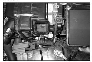
8. Remove the bolt shown that secures the air filter assembly to the mounting bracket.
