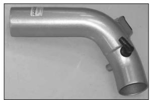
23. Install the 90° barbed fitting into the grommet that was installed into the  $K\&N^{\textcircled{R}}$  intake tube in the previous step.
