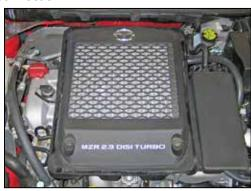
29. Reinstall the engine cover and secure with the factory bolts (removed in step #2).
