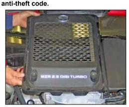
2. Remove the two bolts that secure the intercooler cover, then remove the intercooler cover as shown.
