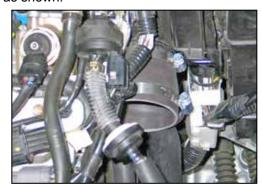
22. Install the provided silicone hose (#084016) onto the turbo inlet with the provided hose clamp as shown.
