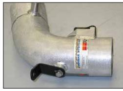
21. Install the tube mounting bracket (#07804) onto the  $K\&N^{\circledR}$  intake tube with the provided hardware as shown.
