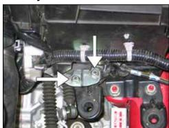
14. Remove the two nuts that secure the wiring harness loom as shown.
