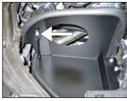
17. Install the heat shield mounting bracket (07945) onto the heat shield with the provided hardware. NOTE: Do not tighten the mounting bracket at this time.
