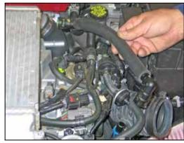
7. Unclip the crankcase vent hose. Remove the complete vent hose as shown.
