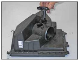
19. Remove the mass air sensor from the stock upper airbox housing as shown.
