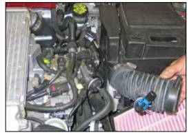
8. Loosen the hose clamp that secures the intake tube to the turbo inlet, then remove the intake tube as shown.
