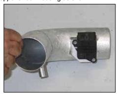
20. Install the mass air sensor into the K&N<sup>®</sup> intake tube with the provided hardware as shown.
