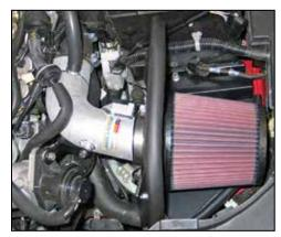
27. Install the K&N® air filter onto the intake tube and secure with the provided hose clamp.
