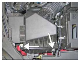
5. Release the two clips that secure the upper airbox housing to the lower airbox housing.
