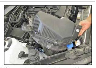
5. Disconnect the factory intake hose and then remove the complete air box assembly from the vehicle.
