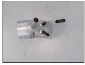
17.Install the provided fittings into the K&N<sup>®</sup> intake tube as shown.
