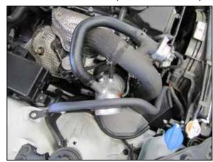
19. Connect the BOV and EVAP hoses to the K&N $^{\circ}$  intake tube.
