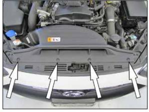
2. Remove the four plastic screws which secure the fresh air intake scoop to the core support and then remove the fresh air scoop from the vehicle.
