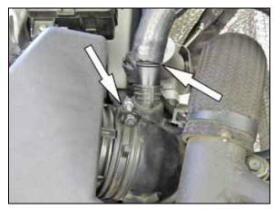
3. Release the spring clamp securing the BOV hose and then disconnect the hose from the factory intake tube. Loosen the hose clamp which secures the factory intake hose to the upper air box.
