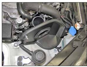
16. Install the heat shield assembly into the vehicle and secure to the rubber mounted stud and fan shroud using the provided hardware.
