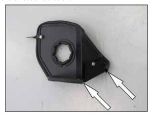
13. Install the 46" section of edge trim around the outside of the heat shield as shown.
