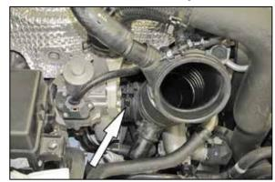
6. Loosen the hose clamp securing the factory intake hose to the turbo inlet. Remove the factory intake hose from the vehicle.
