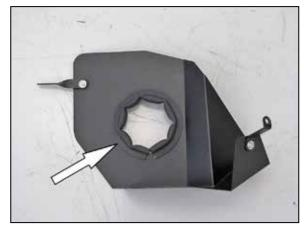
12. Install the 15" section or edge trim into the hole of the heat shield as shown.
