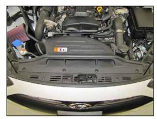
21. Reinstall the fresh air intake scoop and secure with the factory hardware.
