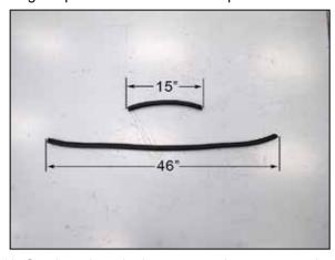
11. Cut the edge trim into two sections, one section will be 15" long and one section will be 46"long.
