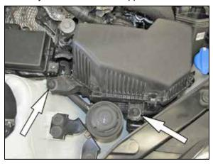
4. Remove the two bolts which secure the factory air box to the inner fender.
