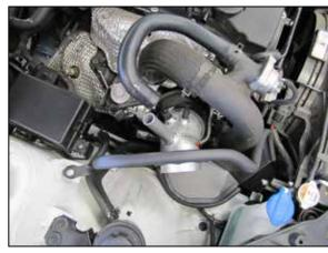
18. Install the K&N® intake tube into the heat shield and silicone hose then adjust the hose and tube for best fit and secure with the provided hose clamps.
