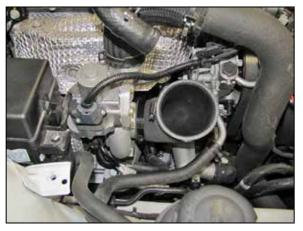
8. Install the provided elbow hose (08504) onto the turbo inlet and secure with the provided hose clamp.
