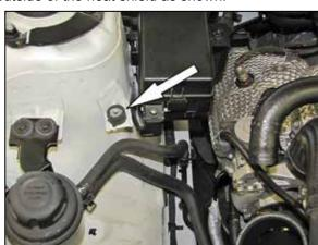
14. Install the provided rubber mounted stud onto the factory air box mounting location on the inner fender.
