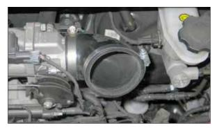
15. Install the provided silicone hose (084087) onto the throttle body and secure with the provided hose clamp.
