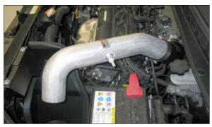
18. Install the K&N® intake tube into the silicone hose at the throttle body and align with the tube mounting bracket. Secure the intake tube with the hose clamp and hardware provided.
