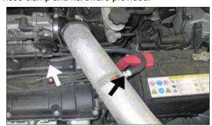
19. Install the provided crank case vent hose onto the 1/4"npt fitting in the K&N® intake tube and then attach the open end to the vent port on the valve
