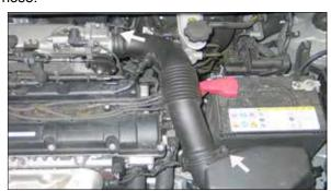
3. Loosen the hose clamps which secure the stock intake tube to the throttle body and air filter housing.
