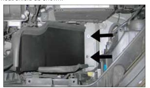
11. Install the heat shield onto the frame rail and secure to the factory stud with the provided hardware and one of the factory air box mounting bolts.
