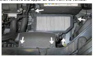
6.Remove the three air box mounting bolts and the two plastic fresh air scoop retaining screws shown.
