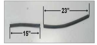
8. Cut the provided edge trim into two lengths, one length of 15" and one length of 23".
