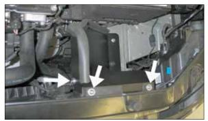
12. Secure the K&N® fresh air scoop to the core support and heat shield using the provided hardware.
