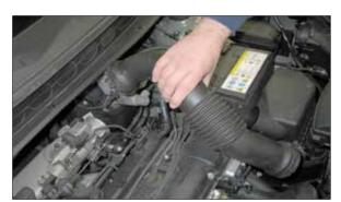
4. Remove the stock intake tube from the vehicle.
