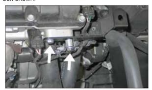
14. Install the K&N® tube mounting bracket (083134) onto the cylinder head and secure with the provided hardware.
