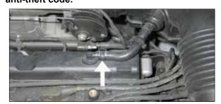
2. Release the spring clamp which secures the crank case vent hose to the valve cover and then unhook the crank case vent hose from valve cover and disconnect the ISC motor wiring harness from the retaining clip attached to the crank case vent hose.
