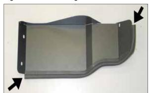
9. Install the 23" long piece of edge trim onto the heat shield as shown.
