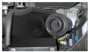
17. Set the K&N® air filter into position at the bottom of the heat shield as shown.
