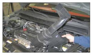
7.Remove the lower air box housing from the vehicle.
