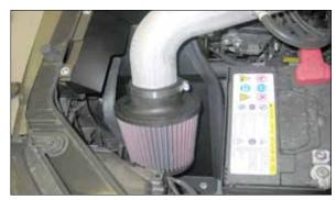
20. Install the K&N® air filter onto the intake tube and secure with the provided hose clamp.
