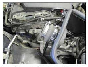
13. Install the provided coupler (087121) onto the filter adapter and secure with the provided hose clamp.
