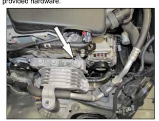
11. Remove the front motor mount bolt shown. **NOTE: This bolt will be reused in the next step.**
