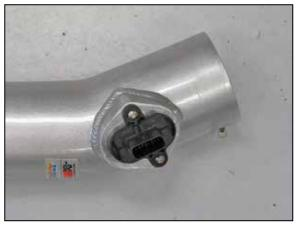
15. Install the mass air sensor into the K&N® intake tube and secure with the provided hardware.
