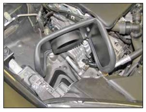
12. Using the factory bolt from the previous step, install the heat shield and spacer onto the motor mount as shown.
