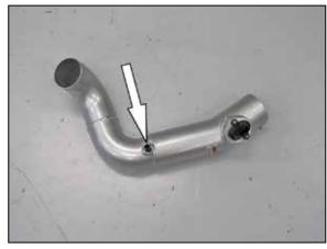
16. Install the provided vent fitting into the K&N® intake tube as shown.
