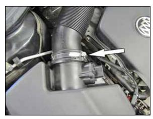
3. Loosen the hose clamp that secures the intake hose to the air filter housing.
