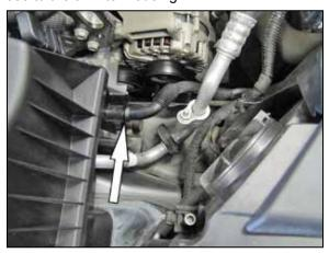
4. Disconnect the air filter housing drain.
