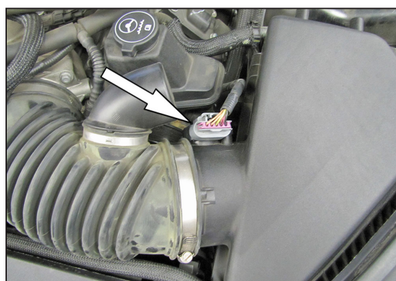
4. Disconnect the mass air sensor electrical connection.
