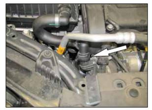
3a. On vehicles that are equipped with air injection, disconnect the air injection hose from the air pump. NOTE: to unlock the air injection fitting, squeeze the outer locking ring to disengage the locking tabs. 4. Lift up and remove the air box from the vehicle as shown.
