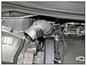
14. Install the K&N<sup>®</sup> intake tube into the silicone hose but do not completely tighten at this time.
