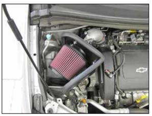
17. Install the K&N<sup>®</sup> air filter onto the intake tube and secure with the provided hose clamp. NOTE: Drycharger<sup>®</sup> air filter wrap; part # RX-4990DK is available to purchase separately. To learn more about Drycharger<sup>®</sup> filter wraps or look up color availability please visit http://www.knfilters.com<sup>®</sup>.
