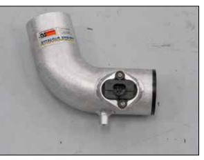
12. Install the mass air sensor into the K&N $^{\mbox{\tiny ®}}$  intake tube and secure with the provided hardware.
