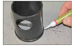
9. Apply several drops of the provided "Super Glue" to the lip of the venturi as shown.
