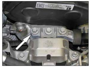
13. Remove the rear engine mounting bolt shown. **NOTE: This bolt will be reused.**
