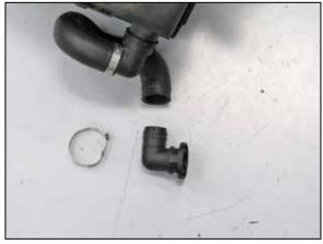
18a. On vehicles equipped with air injection, release the clamp securing the factory air injection fitting to the hose and then remove the fitting from the hose.
