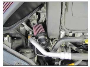
18c. On vehicles equipped with air injection, install the breather assembly onto the air injection pump as shown.
