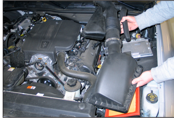
6. Remove the upper air box and intake tube assembly from the vehicle.
