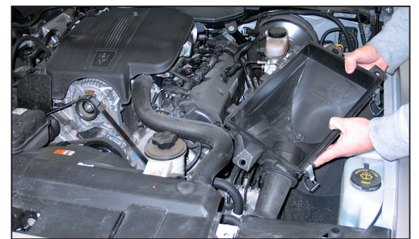
8. Remove the lower air box assembly from the vehicle.
