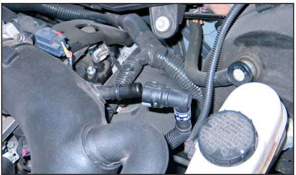
3. Disconnect the crank case vent hose from the intake tube.
