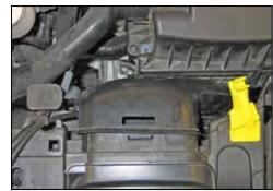
6. Disconnect the fresh air intake scoop from the core support.
