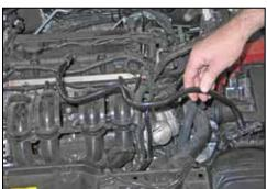
5. Release the locking collar for the crankcase vent hose to the airbox connection by pulling it back, so the crankcase vent hose can be disconnected from the airbox. Then disconnect the crankcase vent hose from the valve cover and remove it from the
