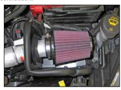
32. Install the K&N® air filter and secure with the provided hose clamp.
