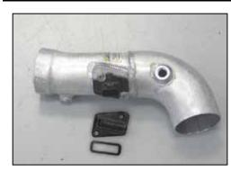
26. On vehicles that are equipped with a mass air sensor install the sensor into the K&N® intake tube and secure with the provided hardware. On all other vehicles, install the provided gasket onto the block off plate and install the block off plate into the K&N® intake tube and secure with the provided hardware.
