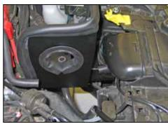
24. Install the fresh air scoop into the scoop attached to the heat shield and then reattach to the factory connection on the core support.
