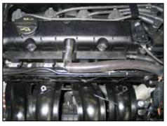
22a. **Non US models:** Install the provided  $\frac{1}{2}$ " silicone vent hose onto the  $\frac{1}{4}$ " vent and guide it along the fuel line towards the intake tube.
