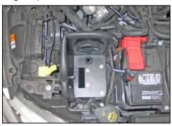
18. Install the heat shield assembly onto the vehicle so that the mounting studs are inserted into the factory mounting grommets, and then secure to the mounting bracket installed during step #10 with the provided hardware.
