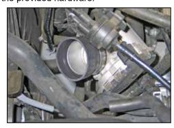
19. Install the provided silicone hose (08476) onto the throttle body and secure with the provided hose clamp.
