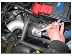
28a. Models without EVAP: Pass the K&N<sup>®</sup> intake tube through the heat shield and rotate so the provided NPT plug (08032) can be installed into the K&N<sup>®</sup> intake tube as shown.
