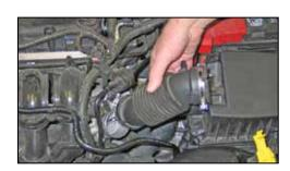
4. Loosen the two hose clamps that secure the factory intake tube and then remove the intake tube from the vehicle
