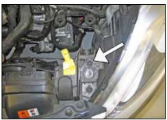
8. Remove the airbox mounting bracket bolt shown.
