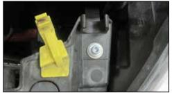
9. Install the provided 30mm long Allen bolt and washer into the air box mounting bracket hole as shown. On some models it may be necessary to use the supplied larger washer.
