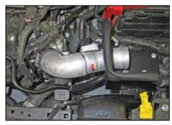
29. When equipped with EVAP, install the K&N® intake tube into the silicone hose at the throttle body and secure with the provided hose clamp. Attach the crankcase vent hose to the installed npt vent fitting.
