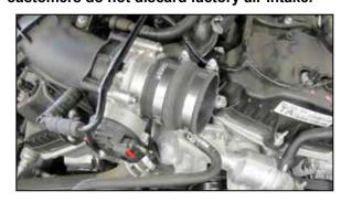
9. Install the provided silicone hose (08696) onto the throttle body and secure with the provided hose clamp as shown.
