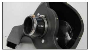
12. Install the provided silicone hose (08724) onto the K&N<sup>®</sup> filter adapter and secure with the provided hose clamp.
