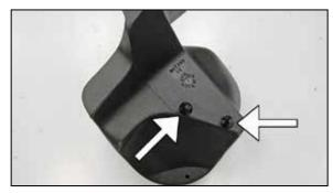
10. Install the two provided mounting studs to the bottom of the K&N® air box as shown and secure with the provided hardware.
