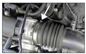
3. Loosen the hose clamp that secures the factory intake tube to the throttle body.
