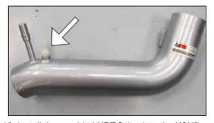
16. Install the provided NPT fitting into the K&N<sup>®</sup> intake tube as shown.
