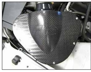
22. Install the air box cover and secure with the provided hardware.
