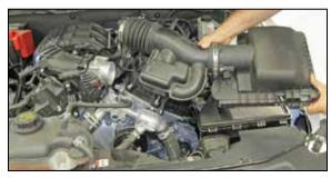
6. Remove the upper air box/tube assembly from the vehicle.
