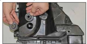
13. Remove the factory air box mounting grommet from the factory lower air box housing.
