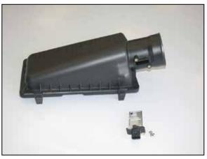
16. Using the "TORX" wrench provided, remove the mass air sensor from the air box lid as shown.
