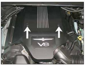
2. Remove the two plastic screws shown securing the engine cover.
