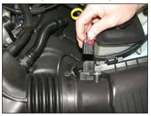
4. Pull back the red locking tab on the mass air sensor electrical connection, and then disconnect the mass air sensor electrical connection.
