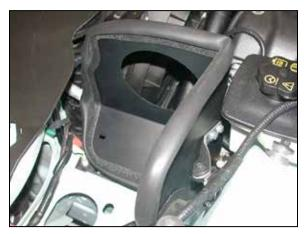
12. Install the heat shield into the vehicle and secure the bracket to the factory air box mount with the factory bolt removed in step #8.
