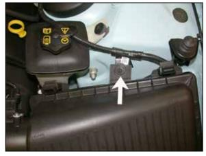
8. Remove the air box retaining bolt shown.
