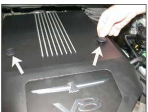
24. Reinstall the engine cover onto the rear retaining clips and then reinstall the retaining clips removed in step #2.
