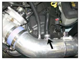
21. Install the large vent hose onto the intake tube as shown.
