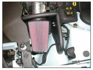
22. Install the air filter and secure with the provided hose clamp.
