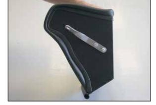
11. Install the heat shield mounting bracket (010083) onto the heat shield as shown with the provided hardware.
