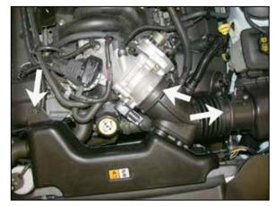
6. Loosen the hose clamps at the throttle body and the factory air box, and then remove the intake tube retaining nut shown.
