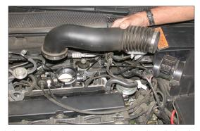
3. Loosen the hose clamps at the throttle body and at the mass air sensor, then, remove the stock intake tube as shown.
