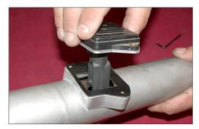
9. Install the mass air sensor into the K&N<sup>®</sup> Typhoon<sup>®</sup> intake tube using the stock bolts from step 8.
