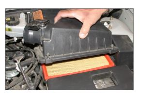
4. Remove the four bolts that secure the air cleaner cover, then remove the cover and filter as shown.
