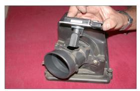
8. Remove the two bolts that secure the mass air sensor, then, remove the mass air sensor as shown.
