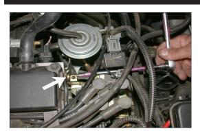
10. Remove the rear bolt on the ignition bracket as shown.
