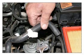
5. Remove the vent hose from the side of the lower air cleaner and valve cover.
