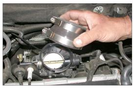
7. Install the provided silicone hose and hose clamps onto the throttle body as shown.
