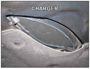
19. Install the guard so the mounting tabs are between the hood and the factory grid as shown.
