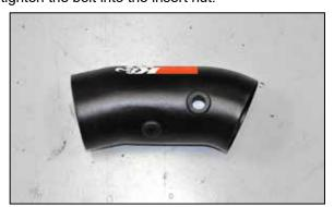
11. Install the two provided grommets into the  $K\&N^{\otimes}$  intake tube.
