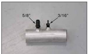
14. Install the 3/16" vent fitting and 5/8" vent fitting into the K&N® intake tube as shown.
