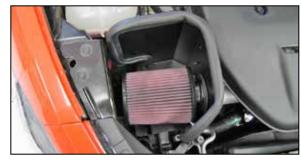
20. Install the K&N® air filter and secure with the provided hose clamp.
