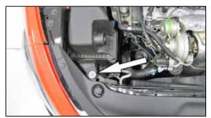
5. Remove the bolt securing the factory air box and then remove the factory air box from the vehicle.
