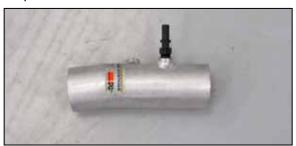
13. Install the provided quick disconnect fitting into the K&N® intake tube as shown.
