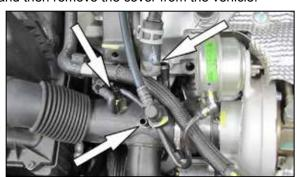
3. Disconnect the crankcase vent hose, EVAP hose and BOV valve hose from the stock intake tube as shown.
