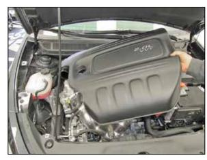
7. Lift up and remove the intake plenum from the vehicle.
