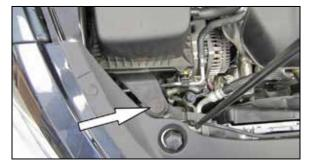
4. Remove the bolt securing the air filter housing onto the core support and unhook the coolant line from the air box.
