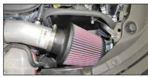
23.Install the K&N® air filter and secure with the provided hose clamp.
