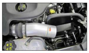
22. Connect the crank case vent hose to the fitting installed into the K&N® intake tube.
