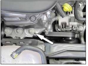
16. Remove the front engine mounting bolt shown.
