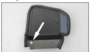
12. Install one of the provided brackets #070812 onto the heat shield as shown using the provided hardware.
