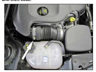
2. Loosen the hose clamp securing the intake hose to the intake plenum.
