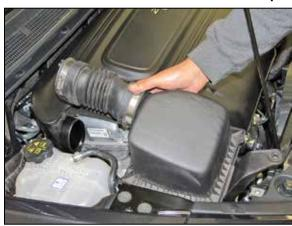
5. Lift up and remove the air filter housing assembly from the vehicle.
