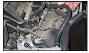
20. Install the provided crankcase vent hose onto the vent port on the valve cover and then connect the open end to the fitting installed into the K&N® intake tube. Some trimming of the crankcase vent hose may be necessary.
