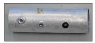
16. Install the provided grommet into the K&N<sup>®</sup> intake tube as shown.
