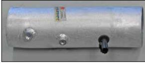
17. Install the inlet air temperature sensor into the grommet installed in the previous step.
