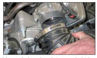
4. Loosen the hose clamp that secures the intake tube to the throttle body and pull the intake tube off of the throttle body.
