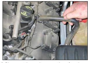
5. Disconnect the crankcase vent hose from the valve cover port as shown.
