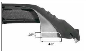
25a. It may be necessary on some vehicles to trim the engine cover as shown to clear the tube mounting bracket.
