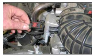
3. Release the red locking tap and then disconnect the inlet air temperature sensor electrical connection.
