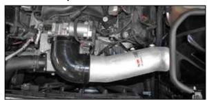
19. Install the K&N® intake tube into the silicone hose at the throttle body and align with the heat shield and mounting bracket. Secure the intake tube with the hose clamp and hardware provided.
