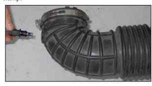
15. Remove the inlet air temperature sensor from the stock intake hose as shown.
