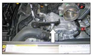
8a. On vehicles equipped with an intake resonator, remove the nut shown which secures the resonator bracket and then remove the resonator bracket from the engine.
