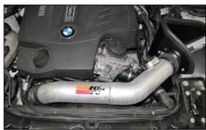
16. Install the K&N® intake tube into the factory turbo inlet tube and then into the filter adapter coupler hose. Adjust the tube and heat shield for best fit and then secure the hose clamps and heat shield hardware.
