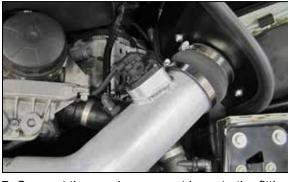
17. Connect the crank case vent hose to the fitting installed into the K&N® intake tube and reconnect the mass air sensor electrical connection.
