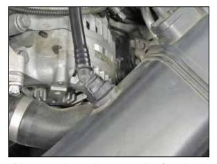
3. Disconnect the crank case vent line from the port on the factory intake tube.
