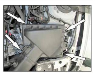
5. Release the four clips securing upper air filter housing to the lower housing. Lift off and remove the intake tube/air filter housing and factory air filter.
