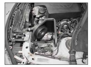
12. Set the heat shield into position so the mounting stud engages with the factory air filter housing mounting grommet and aligns with the fresh air intake duct, secure the fresh air intake duct with the provided hardware but do not completely tighten at this time.
