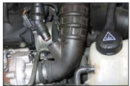
3. Disconnect the crankcase vent hose from the intake tube as shown.
