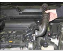
5. Remove the stock intake tube from the vehicle. NOTE: K&N Engineering, Inc., recommends that customers do not discard factory air intake.
