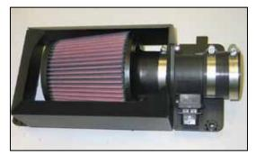
11. Install the provided silicone hose (08440) onto the mass air sensor and secure with the provided hose clamp.
