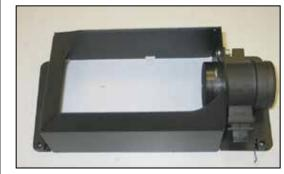
9. Install the mass air sensor into the heat shield and secure with the provided hardware.
