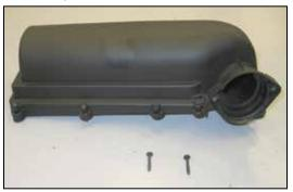
12. Remove two of the upper airbox mounting screws from the upper airbox.
