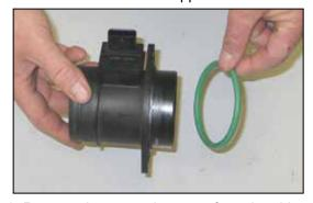
8. Remove the mass air sensor from the airbox, and then remove the "O" ring gasket from the mass air sensor.
