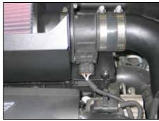
17. Reconnect the mass air sensors electrical connection.
