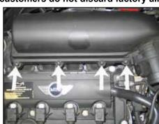
6. Loosen the four screws which secure the upper airbox to the lower airbox, then remove the upper airbox and air filter from the vehicle.
