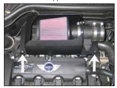
13. Install the heat shield assembly onto the lower airbox. Secure the heat shield assembly to the lower airbox with the two screws removed from the upper airbox in step #12.
