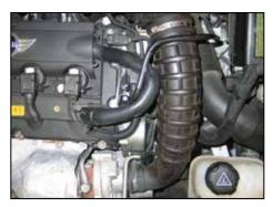
4. Loosen the two hose clamps which secure the intake tube to the turbo inlet and airbox.
