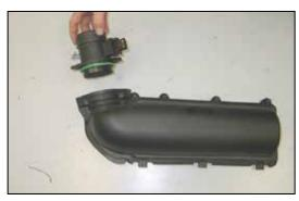
7. Remove the two screws which secure the mass air sensor to the upper airbox and then remove the mass air sensor from the upper airbox.
