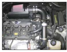
15. Install the K&N® intake tube into the silicone hoses on the turbo inlet and mass air sensor and then secure with the provided hose clamp.
