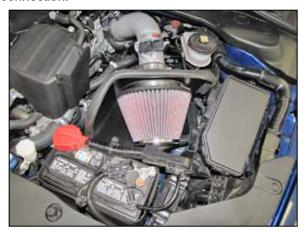
23. Install the K&N® air filter and secure with the provide hose clamp.
