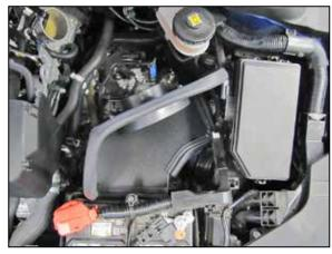
15. Install the heat shield into the vehicle so that the grommet slides onto the mounting stud and the front lines up with the rubber mounted studs. Secure the heat shield with the provided hardware and secure the transmission vent line to the clip installed into the heat shield.
