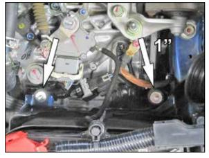
12. Install the two provided rubber mounted studs into the factory air filter housing mounting locations. NOTE: The longer 1" mounting stud is to be installed into the outer most location.
