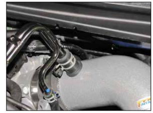
21. Insert the crankcase vent tube into the grommet installed into the K&N® intake tube and use the factory spring clamp to secure.
