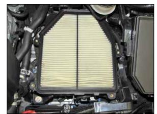
6. Remove the factory air filter.
