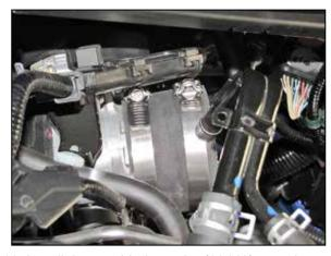
16. Install the provided coupler (08440) onto the throttle body and secure with the provided hose clamp.
