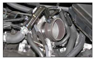
10. Install the provided silicone hose (084014) onto the throttle body and secure with the provided hose clamp.
