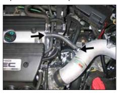
24. Install the provided crankcase vent hose onto the valve cover port and then to the vent fitting on the K&N® intake tube.
