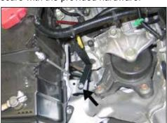
16. Install the front heat shield bracket (070123) onto the lower front air box mounting location using the provided hardware.
