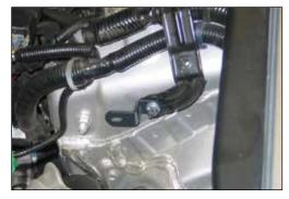
15. Install the heat shield mounting bracket (070061) onto the air box mounting bracket and secure with the provided hardware.
