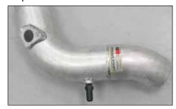
20. Install the provided vent fitting into the K&N<sup>®</sup> intake tube as shown.
