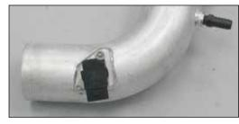
22. Install the mass air sensor into the K&N<sup>®</sup> intake tube and secure with the provided hardware.
