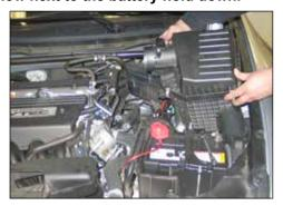
8. Remove the complete air box assembly from the vehicle.
