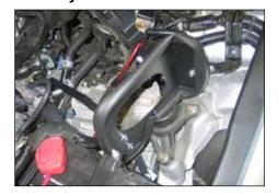
18. Install the heat shield assembly into the vehicle and secure to the mounting brackets with the provided hardware.
