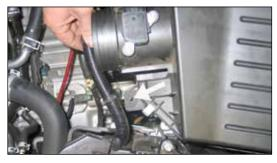
6. Unhook the wiring harness from the air box as shown.
