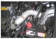
23. Install the K&N® intake tube into the silicone hose at the throttle body and align with the tube mounting bracket installed in step #13. Secure with the provided hose clamp and hardware.
