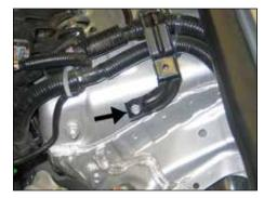
14. Remove the rear air box mounting bracket bolt shown.
