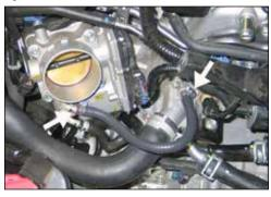
11. Install the provided coolant bypass hose onto the throttle body and thermostat housing and secure with the provided hose clamp.
