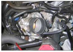
19. Install the provided silicone hose (084036) onto the throttle body and secure with the provided hose clamp.
