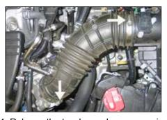
4. Release the two hose clamps securing the intake tube to the air box and throttle body.
