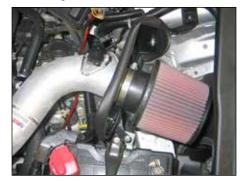
25. Install the  $K\&N^{\otimes}$  air filter and secure with the provided hose clamp.
