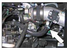
21. Install the provided crankcase vent hose onto the fitting installed onto the K&N® intake tube and then connect the open end to the valve cover vent port.
