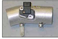
19. Install the provided 90°npt fitting into the K&N<sup>®</sup> intake tube as shown.
