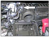
6. Release the spring clamp which secures the crank case vent hose to the air box and then disconnect the crankcase vent hose.
