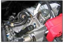
10. Remove the bolt which secures the ground strap to the transmission mount.
