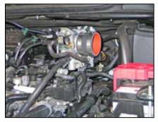
16. Install the provided silicone hose (08284) onto the throttle body and secure with the provided hose clamp.
