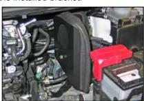
12. Install the heat shield assembly into position and secure to the previously installed bracket with the hardware provided.
