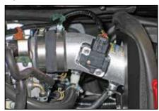
23. Reconnect the mass air sensor electrical connection.
