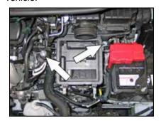
4. Remove the two air box mounting bolts shown.
