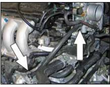
15. Install the provided coolant bypass hose and secure with the provided hose clamps. Be sure to replace any lost coolant.
