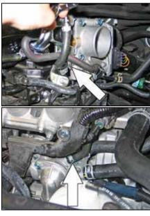
14. Be sure the engine is cool and the cooling system is not under pressure. Loosen the hose clamps and remove the coolant bypass hose from the throttle body and thermostat housing. Be sure to capture any lost coolant in an appropriate container.
