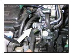
13. Release the spring clamp which secures the crank case vent hose to the valve cover and disconnect the vent hose from the valve cover.
