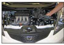
7. Remove the complete air box assembly from the vehicle.
