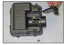
17. Remove the two screws securing the mass air sensor to the air box and then remove the mass air sensor as shown.
