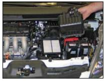
3. Release the four upper air box retaining clips and then remove the upper air box from the vehicle.
