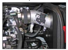
20. Install the K&N® intake tube into the silicone hose on the throttle body and align with the mounting bracket installed onto the heat shield. Secure with the provided hose clamp and hardware.
