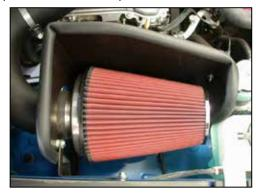
32. Install the K&N® air filter assembly onto the K&N® intake tube and secure with the provided hose clamp.
