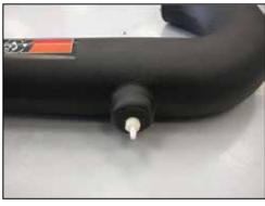
24. Install the supplied 1/4"npt fitting into the K&N® intake tube as shown.
