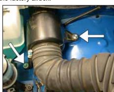
6. Remove the two intake resonator mounting bolts shown.
