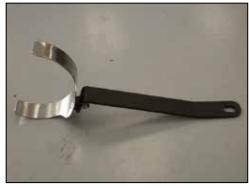
10. Install the saddle clamp onto the tube mounting bracket as shown with the provided hardware.
