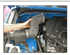
7. Loosen the hose clamp that secures the intake tube to the stock air filter housing, then remove the intake tube and resonator assembly.
