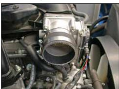
26. Install the silicone hose (08434) onto the throttle body and secure with the provided hose clamp.
