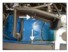
16. Install the heat shield assembly into the vehicle and secure with the provided hardware.
