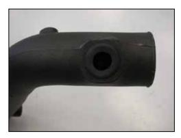
22. Install the supplied grommet into the K&N® intake tube as shown.
