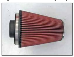
30. Install the supplied filter adapter into the K&N<sup>®</sup> air filter and secure with the provided hose clamp.
