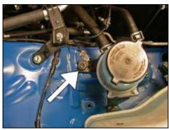
12. Remove the power steering reservoir mounting bolt shown.
