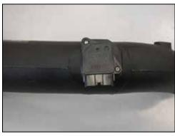
21. Install the mass air sensor assembly into the  $K\&N^{\tiny\textcircled{\tiny 0}}$  intake tube using the supplied hardware.
