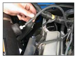
28. Install the supplied fuel pressure regulator vent hose onto the fuel pressure regulator. Attach the opposite end of the vent hose onto the K&N® intake tube as shown.
