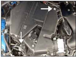
8. Remove the two airbox mounting nuts shown and loosen the hose clamp at the throttle body.
