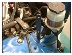
13. Install the "L" bracket onto the power steering reservoir using the bolt removed in step #12. **NOTE: Do not completely tighten at this time.**
