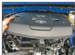
3. Lift up and remove the engine cover.
