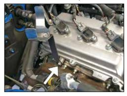
11. Install the tube mounting bracket assembly onto the rear threaded boss on the engine with the provided hardware.
