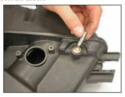
19. Remove the engine cover mounting stud from the airbox as shown.
