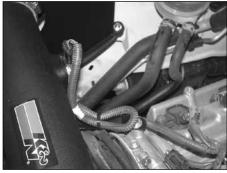
31. Using the provided wire tie, safely secure the excess mass air sensor wiring.
