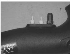
19. Install the provided npt fittings into the intake tube as shown.
