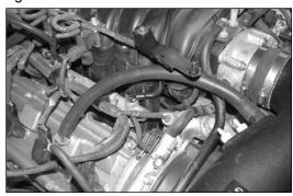
23. Install the provided crankcase vent hose onto the valve cover and then attach to the intake tube as shown.
