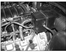
7. Disconnect the three vacuum lines shown from the stock intake tube.
