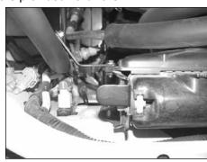
17. Secure the heat shield bracket to the radiator fan shroud with the bolt removed in step #15.
