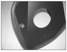
12. Install the rubber mounted studs onto the heat shield as shown using the provided hardware.
