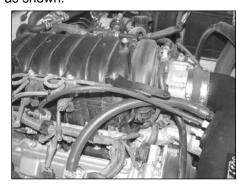
24. Install the provided fuel pressure regulator vent hose onto the fuel pressure regulator and then attach to the intake tube as shown.
