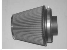
26. Install the filter adapter into the air filter as shown and secure with the provided hose clamp. NOTE: Drycharger® air filter wrap; part number RF-1042DK is available to purchase separately. To learn more about Drycharger® filter wraps or look up color availability please visit http://www.knfilters.com®.
