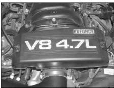
29. Reinstall the engine cover and secure with the nuts removed in step #3.
