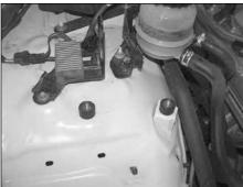
14. Install the two rubber mounted stud to the original airbox mounting holes as shown.
