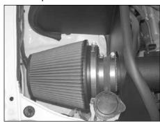
28. Install the air filter assembly onto the intake tube and secure with the provided hose clamp.
