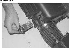
9. Remove the two screws which secures the mass air sensor to the factory airbox, then remove the mass air sensor from the airbox as shown.
