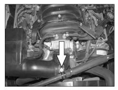
4. Loosen and remove the bolt that secures the A/C hose to the stock intake tube.
