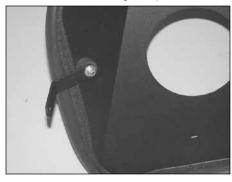
13. Install the provided bracket (070581) onto the rubber mounted stud installed in step #12. Do not tighten completely at this time.
