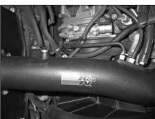
25. Attach the power steering pressure switch vent hose to the intake tube as shown.
