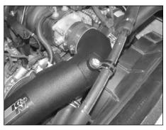
21. Attach the A/C hose to the intake tube with the bolt removed in step #4.
