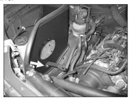
17a. Install the tube mounting bracket (083113) onto the heat shield a shown using the provided hardware.
