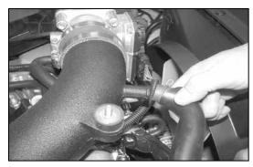
29. Install the original crank case vent hose onto the valve cover, then connect the opposite end of the crank case vent hose onto the K&N® intake tube.
