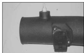
24. Install the vent fitting into the  $K\&N^{\tiny \circledcirc}$  intake tube as shown.
