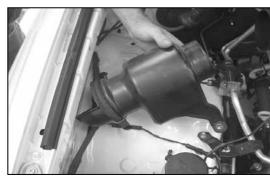
6. Remove the two bolts that secure the resonator to the inner fender, then remove the resonator from the vehicle as shown.
