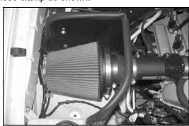
32. Install the K&N® air filter onto the intake tube as shown.
