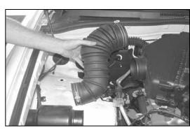
5. Remove intake tube from the vehicle as shown.
