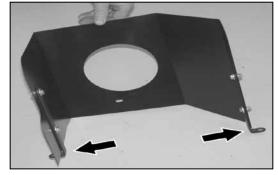
12. Install the two heat shield brackets (07159) onto the heat shield as shown with the provided bardware.
