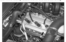
28. Remove the stock vacuum hose from fuel pressure regulator. Attach the provided silicone hose to the fuel pressure regulator and then onto the K&N® intake tube.
