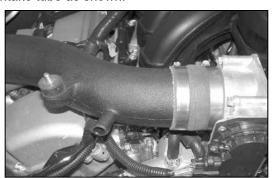
26. Install the K&N® intake tube onto the throttle body and align with the saddle bracket.
