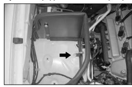
16. Install the heat shield onto the vehicle and secure with the provided hardware and the nut removed in step #15.
