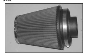
30. Install the radius filter adapter into the air filter and secure with the provided hardware as shown.
