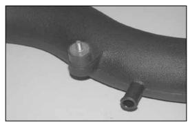
25. Install the rubber mounted stud onto the K&N® intake tube as shown.
