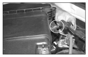
9. Remove the fuel pressure regulator hose from the back side of the air box.
