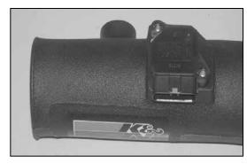
23. Secure the mass air sensor to the K&N® intake tube using the provided screws and spacers as shown.
