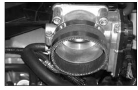
20. Install the silicone hose (08434) onto the throttle body with the provided hose clamps as shown.
