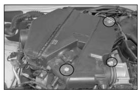
10. Loosen the hose clamp at the throttle body, then remove the two bolts that secure the air box to the engine.
