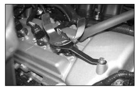
19. Install the tube mounting bracket assembly onto the valve cover with the provided hardware as shown.
