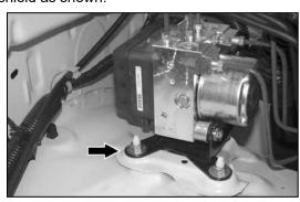
15. Remove the ABS pump mounting nut shown. NOTE: This nut will be reused. Some vehicles may not be equipped with the ABS pump.
