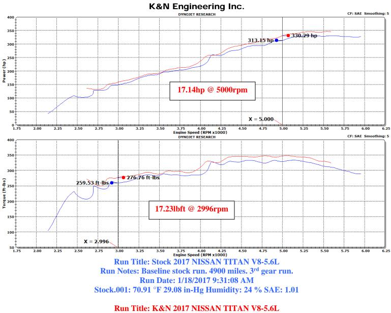
Run Notes: K&N intake kit #63-6019 installed. 4900 miles. 3<sup>rd</sup> gear run. Run Date: 1/18/2017 10:46:54 AM K&N.002: 77.37 °F 29.12 in-Hg Humidity: 20 % SAE: 1.01
