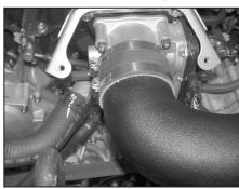
24. Install the K&N® intake tube onto the throttle body and align with the saddle bracket.
