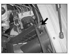
7. Remove the air box mounting bolt with a 10mm socket.
