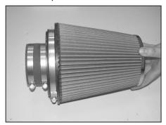
29. Install the filter adapter assembly into the K&N<sup>®</sup> air filter.
