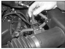
3. Disconnect the mass air sensor electrical connection, then release the wire loom from the air
