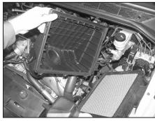
6. Release the two air box lid retainer clips that secure the air box lid to the air box, then remove the air box lid and air filter.
