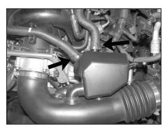
4. Remove the two vent lines from the air intake resonator as shown.
