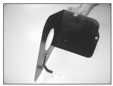
11. Install "L" bracket (07190) onto the heat shield as shown.
