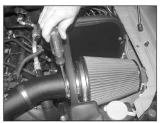
30. Install the K&N® air filter assembly onto the K&N® intake tube as shown; secure with the provided hose clamp.
