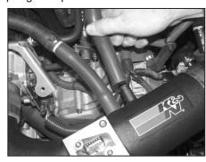
27. Install the provided silicone hose onto the hose mender, then install the hoses onto the intake tube as shown.
