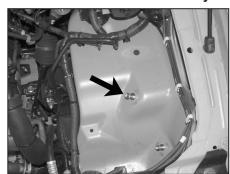
9. Remove the air box mounting stud shown with a 10mm wrench.
