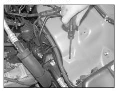
13. Using a screw driver, push the center of the plastic inner fender retaining clip through, then remove the clip from the inner fender.
