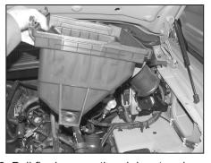
8. Pull firmly up on the air box to release it from the mounting studs, then remove the air box from the
