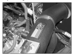
25. Secure the K&N® intake tube to the saddle bracket with the provided hose clamp. Also tighten the hose clamp at the throttle body.
