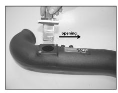
22. Install the mass air sensor assembly into the intake tube with the opening of the sensor pointing towards the air filter end of the tube as shown.
