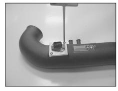
23. Secure the mass air sensor assembly onto the K&N® intake tube with the provided hardware.
