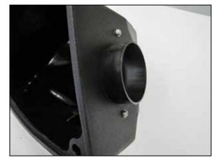
10. Install the provided radius filter adapter into the K&N® air filter housing and secure with the provided hardware.
