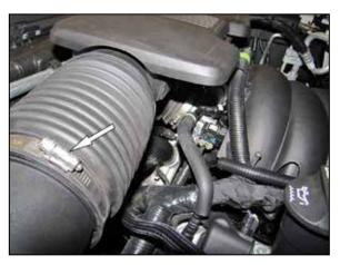
4. Loosen the hose clamps that secure the intake plenum assembly to the throttle body and air filter housing. Disconnect the plenum from the air filter housing and then rotate the plenum assembly counter clockwise to disengage the keyed mount and then remove the plenum from the throttle body. NOTE: Wiring harness anchored to plenum will need to be detached before removing from vehicle.
