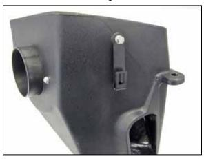
12. Install the provided wiring harness bracket onto the K&N® air filter housing and secure with the provided hardware.
