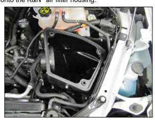
14. Install the K&N® air filter housing into the vehicle so the mounting grommets engage into the factory mounting holes. Secure the housing with the factory nut removed in step #9.
