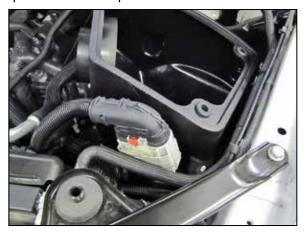
16. Clip the wiring harness onto the bracket installed onto the K&N® air filter housing.
