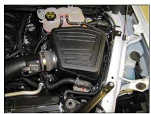
27. Install the K&N® air filter housing lid onto the air filter housing so the posts engage with the mounting grommets.
