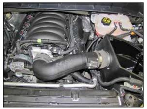
22. Install the K&N® intake tube into the coupler at the air filter housing and then into the coupler on the throttle body, adjust the tube for best fit and then secure with the provided hose clamps.
