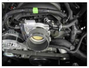
18. On 5.3L vehicles, install coupler #08497 onto the throttle body and secure with the provided hose clamp. On 6.2L vehicles, install coupler #084107 onto the throttle body and secure with the provided hose clamp.
