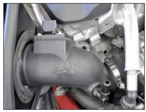
16. Install the K&N® intake tube assembly through the opening in the heat shield and then onto the Turbo inlet. Adjust the tube and heat shield for best fit and then secure them with the hose clamp and hardware.
