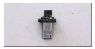
14. Install the mass air sensor into the K&N® mass air sensor adapter and secure with the provided hardware.
