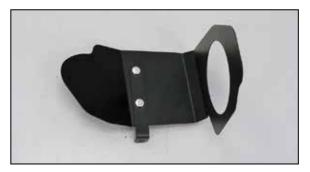
5. Install the heat shield mounting bracket (064337) onto the heat shield as shown using the provided hardware.
