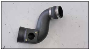
10. Install the provided hump coupler (084018) hose onto the K&N® intake tube and secure with the provided hose clamp.
