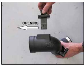
15. Install the mass air sensor assembly into the K&N® intake tube so that the opening in the sensor is towards the air filter end of the intake tube.
