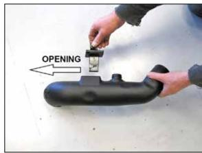
21. Install the mass air sensor assembly into the  $K\&N^{\circledcirc}$  intake tube so that the opening is towards the filter.
