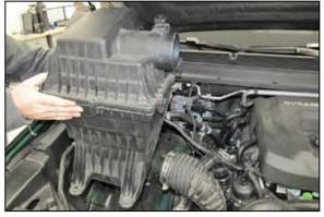
5. Remove the complete air filter housing from the vehicle.
