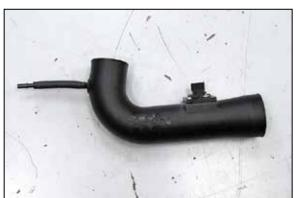
24. Install the EVAP hose assembly onto the K&N® intake tube as shown.
