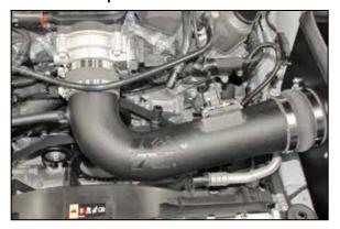
26. Install the K&N® intake tube assembly into the coupler at the filter adapter and then into the coupler on the throttle body, adjust the tube for best fit and then secure with the provided hose clamps.
