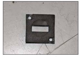
19. Install the gasket on to the  $K\&N^{\tiny{\$}}$  mass air sensor adapter.
