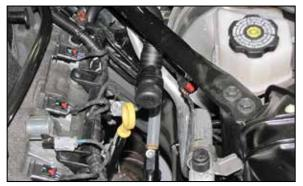
8. Install the caplug assembly into the remaining sound tube and secure with the provided tie wrap.
