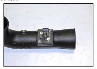
22. Install the mass air assembly into the  $K\&N^{\otimes}$  intake tube as shown.
