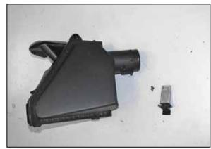
20. Remove the mass air sensor from the factory air filter housing.
