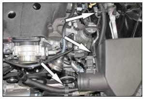
6. Release the three flexible clamps that secure the sound tube and disconnect the sound drum from the rear sound tube then remove the sound tube assembly.
