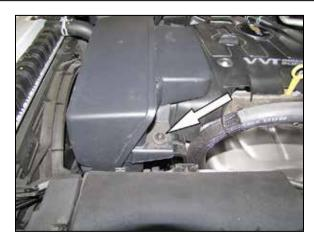
3. Remove the bolt that secures the intake plenum to the engine.
