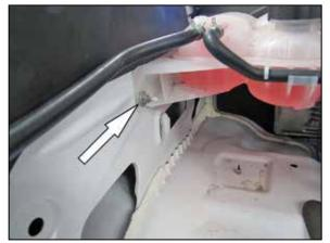
9. Remove the nut securing the coolant reservoir to the inner fender.
