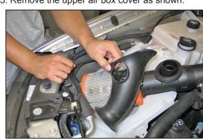
6. Remove the fresh air supply duct.
