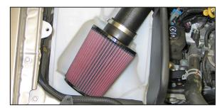
20. Install the K&N® air filter onto the K&N® intake tube and secure with the provided hose clamp. NOTE: Drycharger® air filter wrap; part # RX-4730DK is available to purchase separately. To learn more about Drycharger® filter wraps or look up color availability please visit http://www.knfilters.com®.
