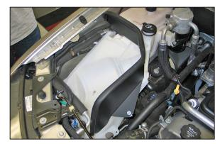
10. Install the heat shield onto the coolant reservoir with the hardware provided.
