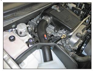
17. Install the K&N® intake tube assembly into the silicone hose at the throttle body and align it with the mounting bracket installed in step #12. Then secure the tube with the provided hose clamp and hardware.
