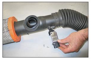
8. Remove the two screws which secure the mass air sensor. Then remove the mass air sensor as shown.
