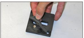
14. Install the adapter gasket onto the adapter plate as shown.
