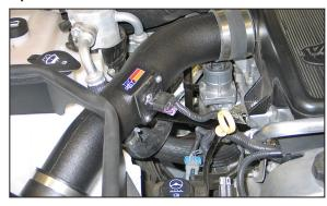
21. Reconnect the mass air sensor electrical connection as shown.
