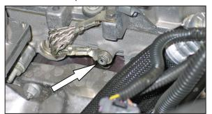
11. Remove the engine ground strap bolt shown. NOTE: This bolt will be reused.
