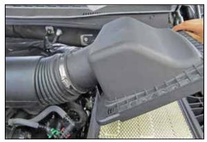
4. Release the locking clips that secure the upper air filter housing to the lower housing, then lift the upper housing and remove it from the vehicle. Remove the factory air filter from the vehicle. 5. Loosen the two hose clamps that secure the factory intake tube to the turbo inlets, then remove the factory intake tube from the vehicle. NOTE: K&N Engineering, Inc., recommends that customers do not discard factory air intake.
