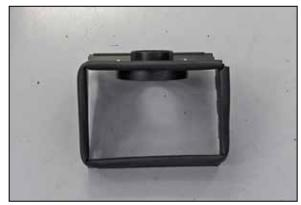
9. Install the K&N $^{\otimes}$  filter adapter into the heat shield and secure with the provided hardware.
