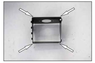
7. Install the small edge trim onto the bottom of the heat shield as shown using the provided super glue to secure it in place.
