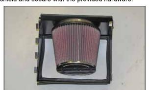
11. Install the K&N® air filter onto the filter adapter and secure with the provided hose clamp.
