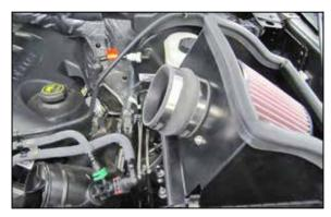
13. Install the provided coupling hose (08699) onto the filter adapter and secure with the provided hose
