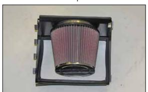
11. Install the K&N® air filter onto the filter adapter and secure with the provided hose clamp. NOTE: Drycharger® air filter wrap; part # RC-5173DK is available to purchase separately. To learn more about Drycharger® filter wraps or look up color availability please visit http://www.knfilters.com®.
