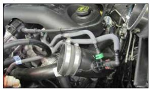
14. Install the provided coupling hose (08761) onto the driver's side turbo inlet tube and secure with the provided hose clamp.
