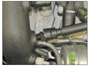
18. Connect the two vacuum lines to the fittings installed into the K&N® intake tube as shown.
