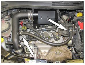
19. Install the provided crank case vent hose onto the plenum and then onto the fitting installed into the K&N® intake tube and secure with the provided hose clamps.
