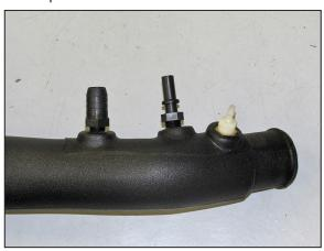
15. Install the three vent fittings into the  $K\&N^{\otimes}$  intake tube as shown.
