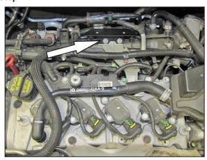
11. Install the heat shield mounting bracket (064321) onto the studs and secure with the factory nuts removed in the previous step.
