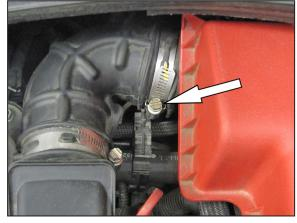
4. Loosen the hose clamp securing the intake hose to the air filter housing.
