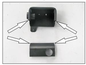
13. Install the 17-1/2" long section onto the heat shield and the 8-3/4" long section as shown.
