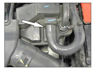
7. Disconnect the crank case vent hose from the plenum where shown.
