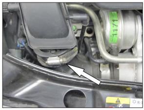
2. Loosen the hose clamp securing the turbo inlet hose to the plastic intake tube.
