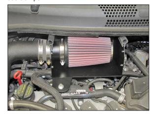
20. Install the K&N® air filter onto the heat shield tube and then secure with the provided hose clamp.
