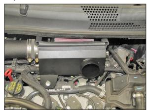
21. Install the heat shield cover and secure with the provided hardware.
