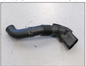
24. Install the K&N® fresh air intake tube into the factory fresh air duct as shown.
