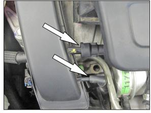
3. Disconnect the vacuum line and crank case vent hose from the plastic intake tube.
