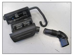
23. Remove the fresh air duct from the factory air filter housing as shown.
