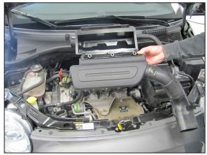
9. Lift up the air box housing to unhook it from the mounting studs and then remove the intake housing from the vehicle.
