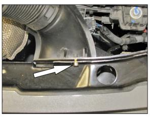
8. Remove the bolt securing the fresh air intake duct to the core support.
