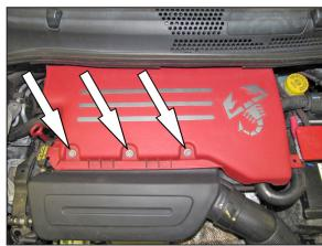
6. Loosen the three screws and remove the air filter housing lid and air filter.
