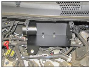
14. Install the heat shield onto the K&N® mounting bracket and the factory engine bracket and secure with the provided hardware.
