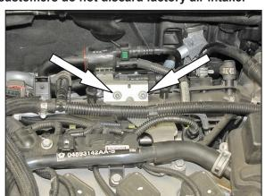
10. Remove the two nuts shown securing the reinforcement bracket to the intake manifold. **NOTE: These nuts will be reused in the next step.**
