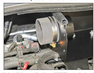
16. Install the coupling hose (08727) onto the heat shield tube as shown and secure with the provided hose clamp.
