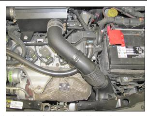
25. Install the fresh air assembly into the core support and then into the hose at the heat shield. Secure the assembly with the factory bolt and hose clamp provided.
