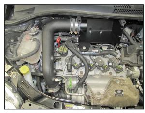
17. Install the K&N® intake tube into the factory turbo intake tube and then into the coupling hose on the heat shield tube. Secure the tube with the provided hose clamps.
