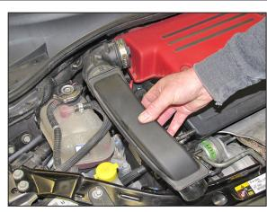
5. Remove the plastic intake tube and coupler as shown.
