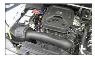
17. Install the intake assembly into the vehicle so the mounting studs insert into the mounting grommets and the intake tube inserts into the coupler. Secure the system with the provided hose clamp and hardware.
