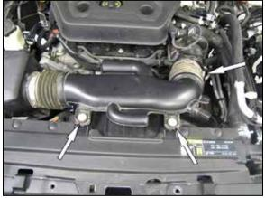
4. Remove the two bolts that secure the intake tube to the core support. Loosen the hose clamp securing the intake tube to the throttle body.
