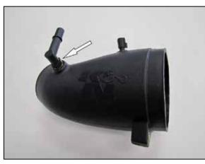
11. Install the provided 90° quick disconnect fitting into the K&N<sup>®</sup> intake tube as shown. **NOTE: Plastic NPT fittings are easy to cross**
