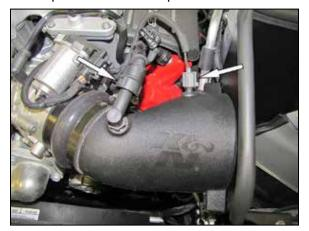
15. Reconnect the inlet air temperature sensor electrical connection. On 2018 DEMON models connect the crank case vent quick connect fitting to the fitting installed into the K&N<sup>®</sup> intake tube. power and performance from your kit.
