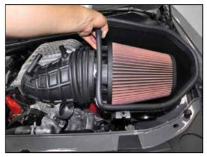
5. Remove the complete factory intake system from the vehicle.
