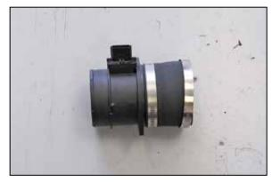
10. Install the provided coupling hose (08496) onto the mass air sensor as shown and secure with the provided hose clamp.
