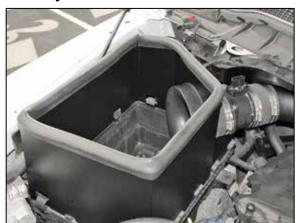
14. Install the heat shield onto the lower air filter housing and secure with the factory retaining clips. NOTE: It is best to install the coupling hose onto the filter adapter as the heat shield is being set into position.
