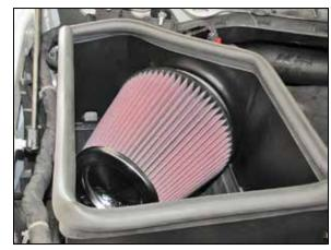
16. Install the K&N<sup>®</sup> air filter onto the filter adapter and secure with the provided hose clamp. NOTE: Drycharger® air filter wrap; part # RF-1042DK is available to purchase separately. To learn more about Drycharger® filter wraps or look up color availability please visit http://www.knfilters.com®.
