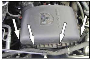
4. Release the four clips securing the upper air filter housing and then remove the housing and air filter
