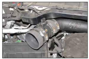
11. Install the mass air sensor into the coupling hose installed onto the K&N® intake tube.
