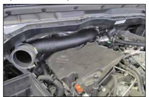
8. Install the  $K\&N^{\otimes}$  intake tube into the factory turbo inlet hose and secure with the factory hose clamp.
