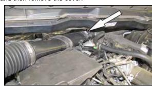
6. Loosen the hose clamp securing the intake tube to the turbo inlet hose. Lift up the intake tube to dislodge it from the mounting stud and then remove the tube from the vehicle.
