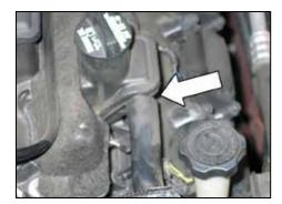
4. Disconnect the crank case vent hose from the valve cover.
