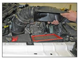
4. Release the two clips securing the air box lid; remove the air box lid and intake tube from the vehicle.
