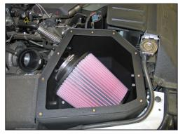
20. Set the K&N® air filter into the K&N® air box as shown.
