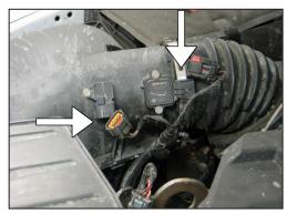
2. Disconnect the mass air sensor and temperature sensor electrical connections, then unhook the wiring harness from the air box.
