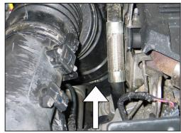
3. Loosen the hose clamp securing the intake resonator to the turbo inlet hose.
