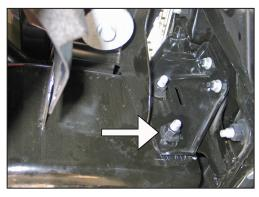
12. Remove the passenger side lower bumper mounting bracket nut shown.
