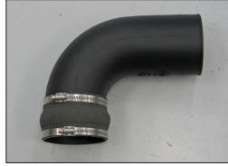
22. Install the provided silicone hose (08695) and hose clamps onto the  $K\&N^{\otimes}$  intake tube as shown. NOTE: Do not completely tighten at this time.
