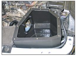
11. Install the air box so the mounting studs insert into the air box mounting grommets, then secure the air box to the mounting bracket that was installed in step #8. Tighten the mounting bracket bolts.
