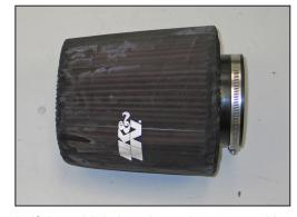
19. If the vehicle is going to be operated in extreme wet or snow conditions, it is recommended that a Drycharger® air filter wrap, sold separately, be installed onto the K&N® air filter.
