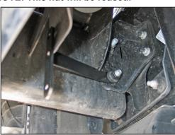
13. Install the tube mounting bracket (083157) onto the stud as shown and secure with the factory nut removed in the previous step.
