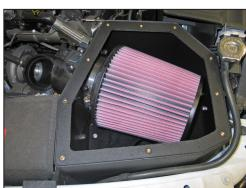
21. Install the K&N® mass air housing onto the mounting studs and into the K&N® air filter inlet. Secure the housing to the studs with the provided hardware and then secure the air filter with the provided hose clamp.
