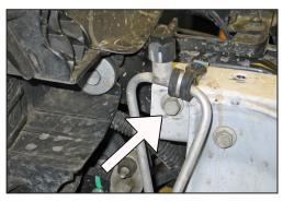
7. Remove the core support bolt shown. **NOTE: This bolt will be reused in the next step.**
