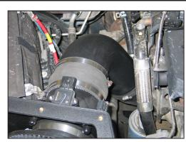
23. Install the K&N® intake tube into the factory turbo inlet hose and then connect the K&N® hose to the K&N® mass air sensor housing. Secure the intake tube with the hose clamps provided.
