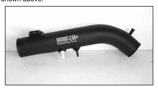
11. Install the provided vents into the K&N $^{\mbox{\tiny 8}}$  intake tube.
