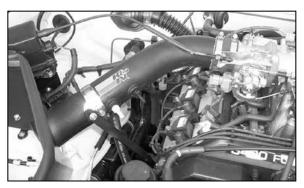
22. Install the K&N® intake tube onto the throttle body then tighten the hose clamps at the throttle body and saddle bracket.
