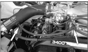
26. Install the new silicone hose onto the K&N® intake tube and then install the other end onto the intake manifold as shown.
