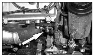
18. Loosen and remove the bolt that secures the wire harness bracket located directly behind the power steering reservoir.
