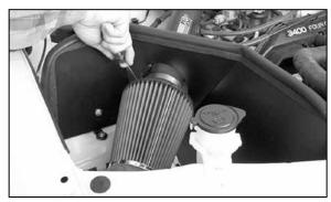
29. Install the K&N® Filter onto the K&N® intake tube and secure it with the provided hose clamp. NOTE: Drycharger® air filter wrap; part # RC-4700DK is available to purchase separately. To learn more about Drycharger® filter wraps or look up color availability please visit http://www.knfilters.com®.
