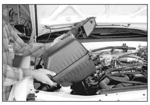
7. Remove the complete air intake system.
