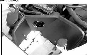
20. Install the heat shield and secure it to the new K&N® brackets with the hardware provided. Do not tighten completely.
