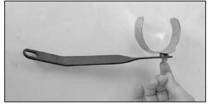
15. Assemble the saddle bracket as shown.
