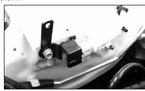
17. Install the bracket onto the relay bracket using the bolt that was removed in step 16. Do not tighten completely.
