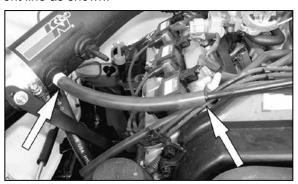
24. Install the provided silicone hose onto the K&N® intake tube and connect the other end to the hard vent line as shown.
