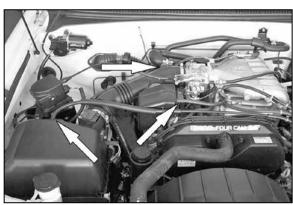
3. Disconnect the three hoses from the air box resonator and intake hose.
