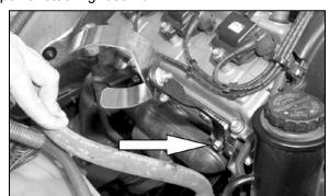
19. Install the saddle bracket assembly onto the motor using the bolt from step 18. Do not tighten completely.
