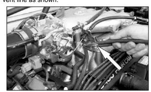
25. Remove the rubber hose from the intake manifold as shown.
