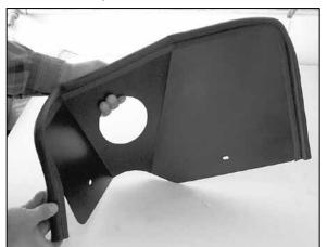
12. Install the edge trim onto the heat shield as shown above. Trim if needed.
