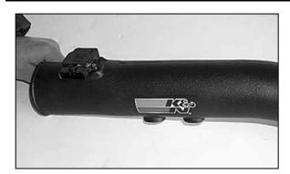
10. Using the provided screws and spacers install the mass air sensor into the K&N<sup>®</sup> intake tube as shown above.
