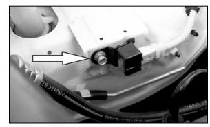
16. Remove the bolt from the relay bracket as shown.
