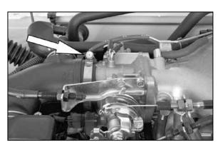
4. Loosen the hose clamp at the throttle body.
