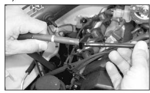
23. Remove the rubber hose from the hard plastic vent line as shown.
