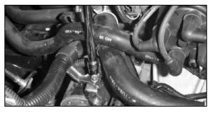
7. Loosen and remove the bolt that secures the wiring harness bracket to it's support bracket. **NOTE: This bolt will not be reused.**
