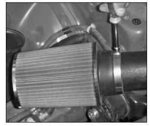
15. Install the Filtercharger element onto the intake tube and secure it with the provided hose clamp.
