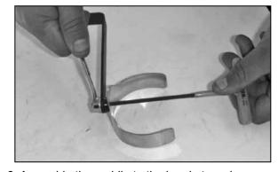
8. Assemble the saddle to the bracket as shown. NOTE: On models with manual trans. use the "L" bracket and on models with auto trans. use the angled "L" bracket.
