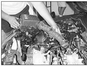
6. Remove the complete air intake assembly as shown.
