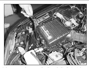
4. Loosen and remove the three bolts that retain the airbox.
