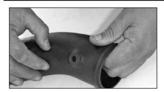
10. Install the grommet supplied into the small hole in the K&N® intake tube.
