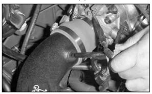
13. Insert the crankcase vent tube into the grommet in the K&N® intake tube.
