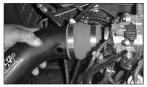
12. Install the intake tube onto the throttle body and secure it with the provided hose clamp.
