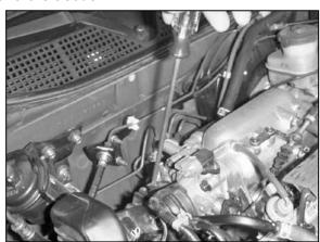
2. Loosen the hose clamp on the intake tube at the throttle body.
