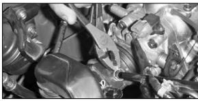
5. Remove the crankcase vent tube from the stock intake tube.
