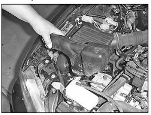
3. Pull firmly upward and remove the air inlet duct.
