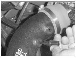
15. Install the air temperature into the grommet on the K&N<sup>®</sup> intake tube.
