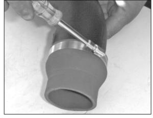
11. Install the silicone adapter onto the K&N<sup>®</sup> intake tube.
