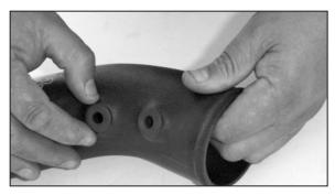
10. Install the grommets supplied into the 2 small holes in the K&N® intake tube.
