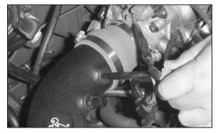
16. Insert the crankcase vent tube into the second grommet on the K&N® intake tube.
