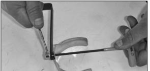
2. Loosen the hose clamp on the intake tube at the throttle body.
