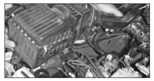
6. Remove the complete air intake assembly as shown.
