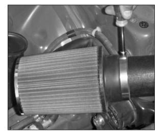
18. Install the Air Filter element onto the intake tube and secure it with the provided hose clamp.
